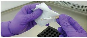
3. Clean the outside of the ampoule using a disinfectant wipe or tissue soaked in 70% alcohol.
