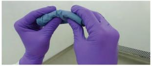
7. Snap the ampoule while wrapped where the score mark was made.
