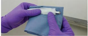
Then wrap with paper towels, tissue or gauze to act as a padding layer. This is to prevent accidental injury when the ampoule is snapped open.
