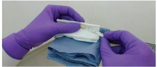
8. Carefully unwrap the ampoule as fragments of glass may be present in the tissue. Discard the tissue and the ampoule tip into a sharps bin.
